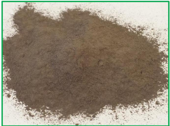
**Finely ground bulk phosphate sample to 100Mesh
